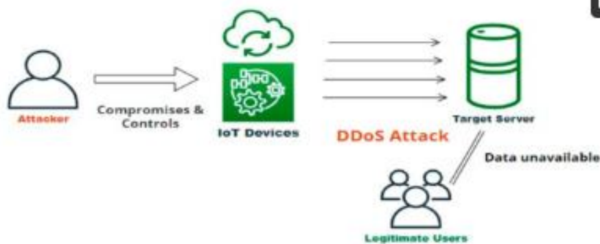
Figure 5. DDoS attack in IoT platform.
